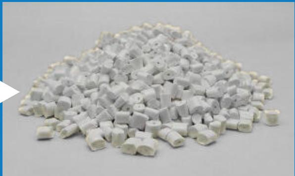
The material is polypropylene, the melting point can be as high as 167°C, Vicat softening temperature of 150°C.
